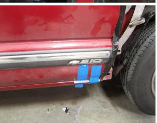
15) New hole pattern on the body and door: Center the hinge and use a "punch" to mark the new hole pattern make sure to me the marks in the middle of the holes so that you have room for adjustments later. Use a 17/64 US Drill or 6.70mm metric to make the new hole pattern for a 8MMx1.25 Tap.
