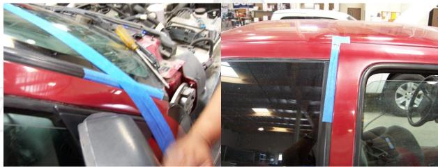
To replace the door make sure to use the marks on the tape (step 11) use blue painters tape to secure the door to the body.
