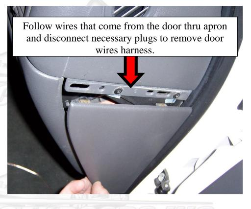
Close the door and remove the factory wire loom and pull the wires out of the body and put them inside the door.
