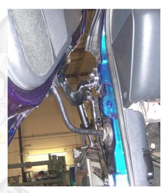
21) You will have to cut the inner lip of your fender to make room for the new Vertical Doors Inc. system.
