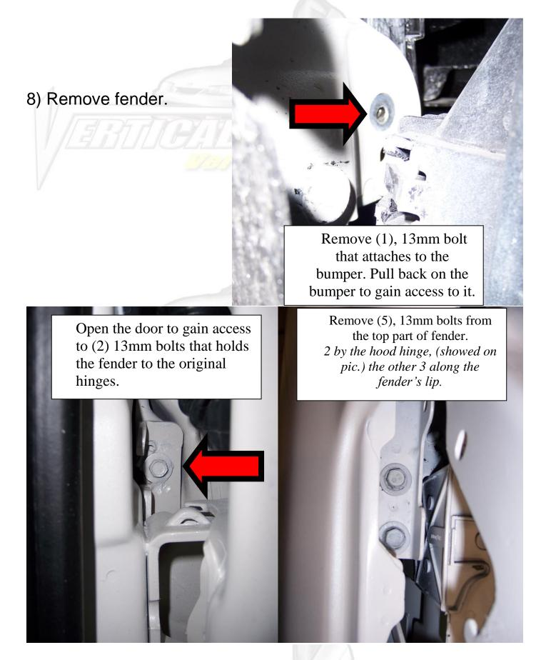
Remove (1) 13mm bolt that is located at the bottom of the bumper by the door.
