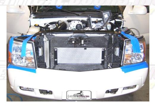
5) Disconnect the Fuse box. There are (4), 10mm bolts securing the fuse box to the fender. (2) of them are Horizontal and (2) of them are Vertical.
